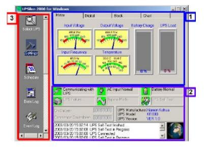
Section 1 is the UPS Dynamic Display Area where relevant information regarding the UPS is displayed. Selection of different display modes is possible, with information including input voltage, output voltage, line frequency, battery capacity, load, temperature, etc.
