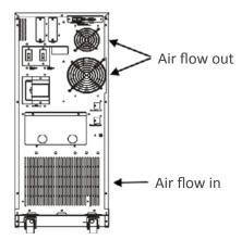
Select an installation position with at least 30 cm around the UPS and Battery bank , where may provide a good ventilation condition as indicated below
