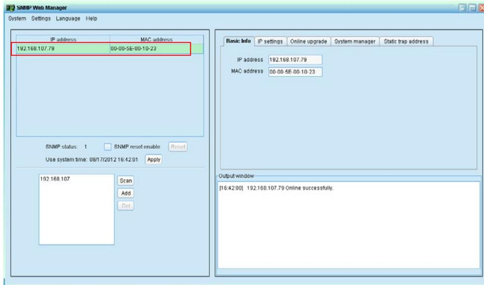
User can modify IP setting, online upgrade, password management, and static trap address setting in SNMP Web Manager interface. It is necessary to enter password for any medications. The default password is 12345678.
