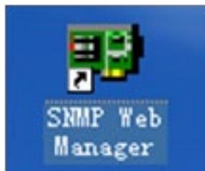
Enter specific IP address to search all SNMP devices in LAN. The SNMP web manager is default applied static IP address as 192.168.102.230, default subnet mask as 255.255.255.0, and default gateway as 192.168.102.1. Users can modify IP address or apply DHCP mode through web server of SNMP web pro card, SSH Client or SNMP Web Manager.
