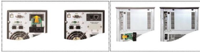
**Step 3:** Plug Ethernet cable to the Ethernet port (RJ-45) on the SNMP web manager.
