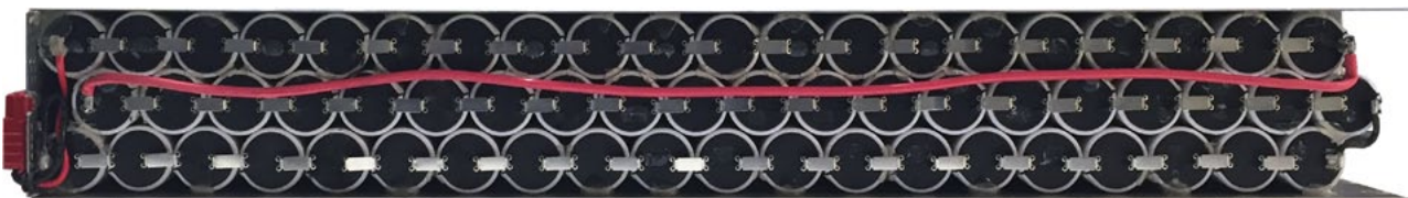
R91-BPSYS battery module connection
