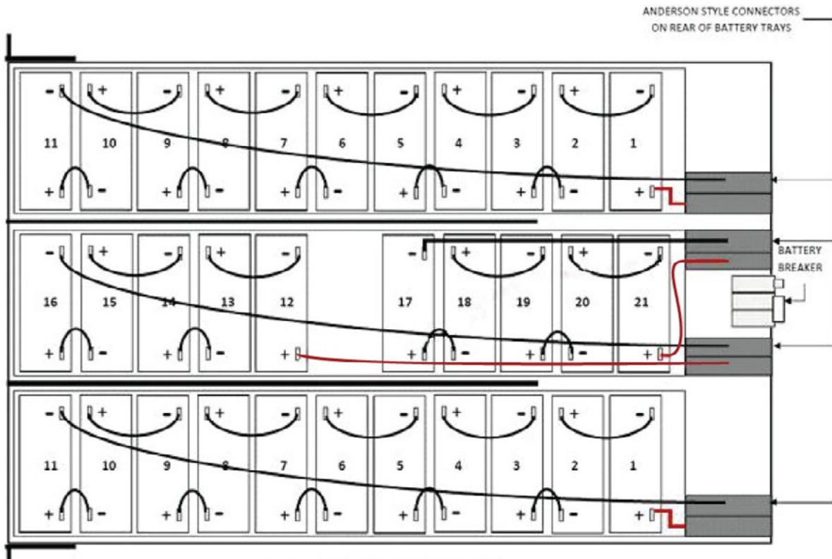
± 192VDC battery connection diagram internal EBP32
