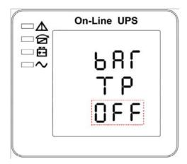
Battery temperature compensation sensor switch setting
