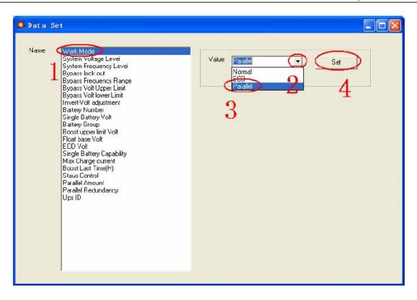
• At the window of "Data Set", select "UPS ID", enter the Value for the parallel UPS ID at the right side, then select "Set" as shown in the figure below. If the UPS "beeps" it means the setting is correct.
