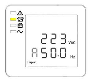
PHASE A (L1) INPUT VOLTAGE / FREQUENCY
