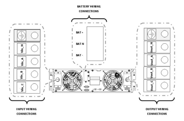
Power cable connection diagram
