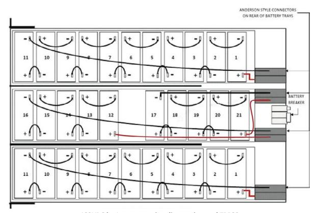
**± 192VDC battery connection diagram internal EBP32**
