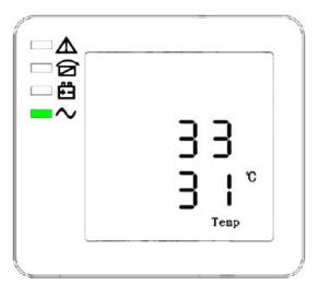
INTERNAL TEMPERATURE AND AMBIENT TEMPERATURE
