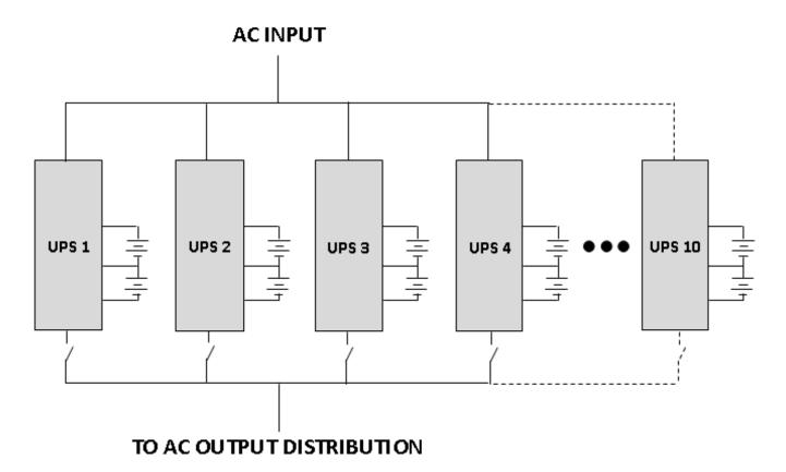
**Note:** If installing 5-6 units in parallel, remove the jumper cap J30 on the control inspection board (MHTBJHR-1CU04 in all UPS to be connected in parallel. If installing 7-10 units in parallel, remove the jumper cap J30/J31 on the control inspection board (MHTBJHR1CU04 in all UPS to be connected in parallel. Make sure that each UPS input breaker is in the "OFF" position and there is no output from any UPS connected. The battery strings can be connected separately or in parallel.
