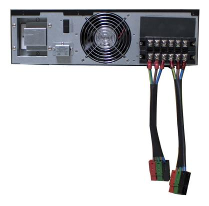
Connect UPS input to utility input terminals on P90L-ISO10MB terminal block with the provided Anderson connectors.
