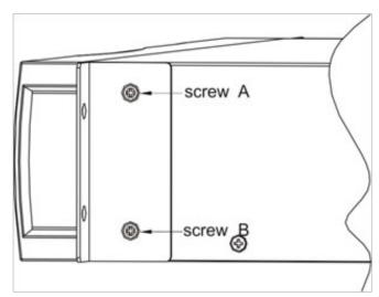
**UPS Front Corner With Bracket Installed**
