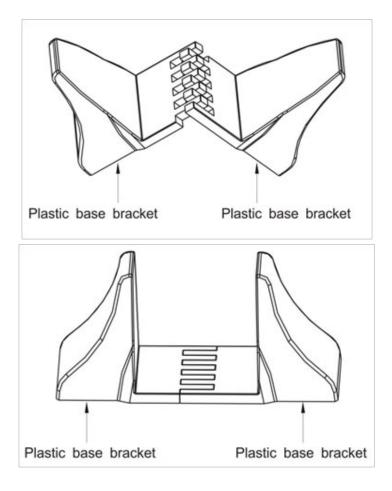
The same plastic base assembly plus a 1U plastic base extension bracket are connected together as shown below to accommodate 3U enclosures.
