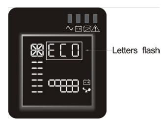
• Enter the ECO setting interface. Press and hold the function setting button for more than ½ second but less than 2 seconds, then come to setting interface of ECO, the letters "ECO" will light for a long time. The "ON" below the ECO will flash. Press and hold the inquiring button for more than ½ second but less than 2 seconds to determine whether the ECO function is used or not. If used, the corresponding word is "ON", if not, the word is "OFF".
