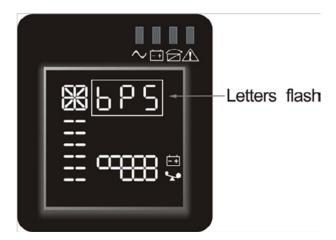
• Enter the Bypass output setting interface. Press and hold the function setting button for more than ½ second but less than 2 seconds, at this time the letters "bPS" will light for an extended period. The "ON" below the bPS will flash. Press and hold the inquiring button for more than ½ second but less than 2 seconds to determine whether the bPS function is used or not. If used, the corresponding word is "ON", if not, the word is "OFF".
