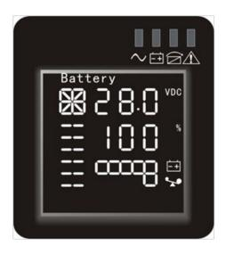
Press and hold the inquiring button for more than 2 seconds, LCD begins to display the items sequentially every 2 seconds. Press and hold the button again and the display will return to output status.
