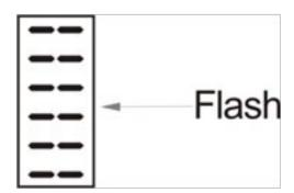
When the UPS is in Battery Mode, the number of icons for the charger status section will vary according to the changeable capacity of the battery. For example, there are five panes in the figure below, so the corresponding number of icons is five rows.
