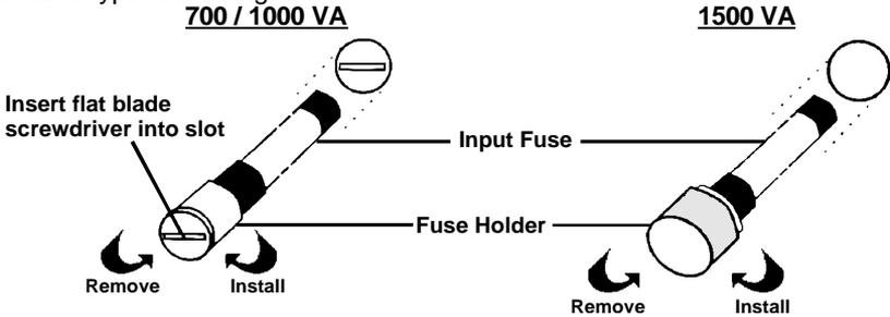
1. Remove the fuse holder by inserting a flat blade screwdriver into the slot (twist by hand for the 1500 VA model) and rotating counter-clockwise to remove.
