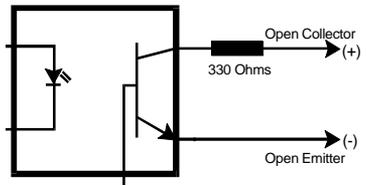
\*Maximum voltage and current on pins 1,7,8,9 is 80V DC; 10.0 mA.
