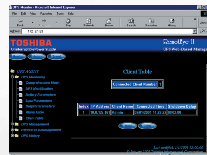
RemotEye II's web interface allows a user to view the protected machines RemotEye II oversees.
