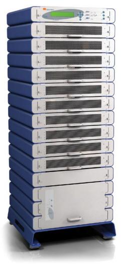
The **Gamatronic Power+ M100** is a parallel redundant modular UPS capable of scaling from 10kVA to 100kVA. Comprised of one to ten 10kVA/8kW UPS modules, as well as a system controller, a 100kVA static switch, and a distribution block, the system easily grows with your requirements.
