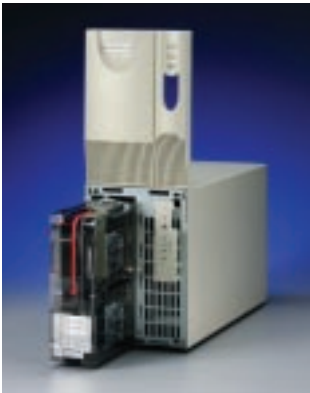
Powerware 5125 shown with front cover removed and battery out.
